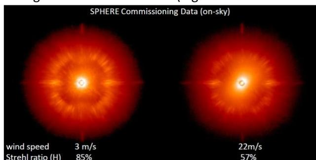
**Figure 1:** Impact of the AO temporal error on VLT/SPHERE coronagraphic images. Left: under slow evolving turbulence. Right: under fast evolving turbulence (contrast decreased by one magnitude).
